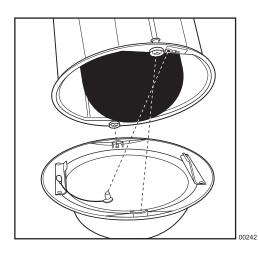
Figure 1. Lower Dome Installation, In-Ceiling Models
